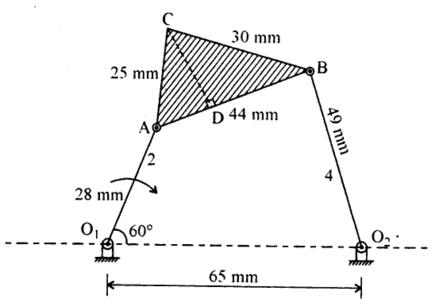
$O_1O_2 = 65 \text{ mm}, O_1A = 28 \text{ mm}, O_2B = 49 \text{ mm}, AB = 44 \text{ mm},$
