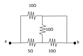
3. Calculate value of I<sub>N</sub> for the circuit shown in Fig.
