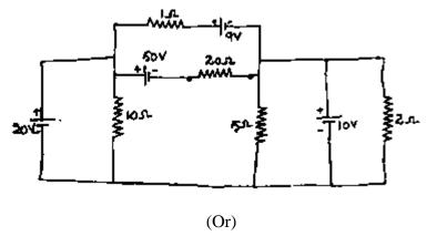
(b) Find the current through 5 ohm resistor using superposition theorem in the circuit shown in Fig. (16)
