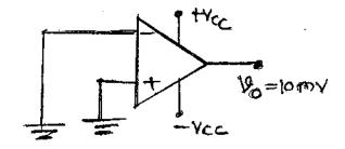
d) What output voltage results in the following circuit for an input voltage
